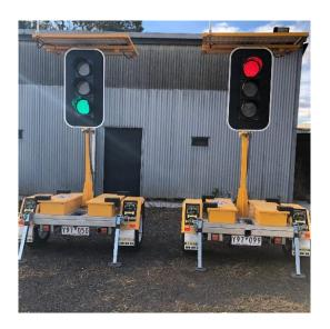
The master is the WIFI access point and the slave is the WIFI station. The two stations cooperate together. When the green cycle has finished in one, it is going to message to the other. The other is doing same. To test their behavior at the same time you have to go to the simulator folder and start E32MT.exe multitester. The multitester appears at the top of the screen. You have to left click on its surface.
